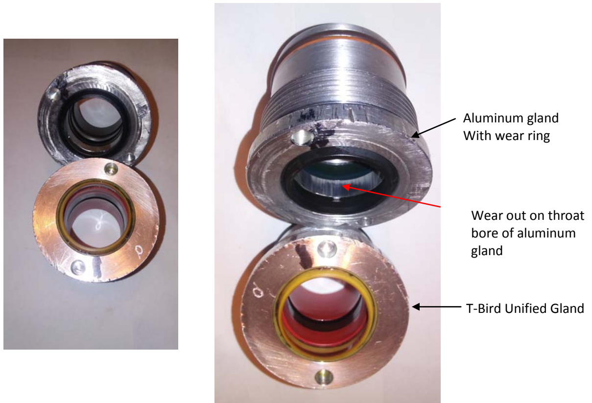
Figure 4: T-Bird Unified Gland after 800,000 strokes versus Aluminum gland with wear ring after 400,000 strokes
